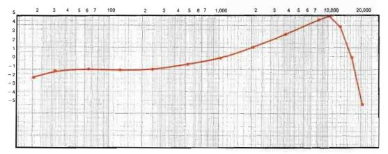
Figure 2. Equalization curve used in disc-to-cart music transfer.
