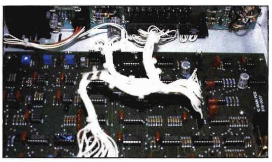
The rows of relays and shunt resistors common in the control/overload circuits of older transmitters are being replaced by integrated circuit logic gates and microprocessor chips. These high-tech designs have allowed additional features to be built into transmission equipment, greatly simplifying troubleshooting.
