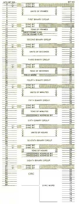
Vertical interval time code contains 90 bits of information. The additional data aids "housekeeping" chores and provides field, rather than frame, edit capability.
