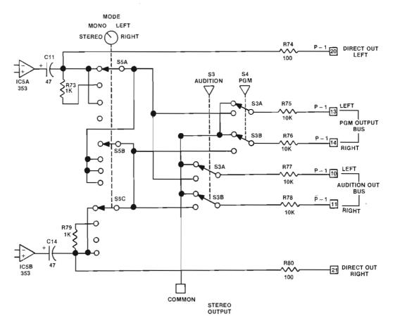
Figure 1. Output wiring for standard Auditronics monaural (upper) and stereo line-level (lower)
