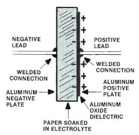
Figure 20. The basic design of an aluminum electrolytic capacitor. (Reference 32.)
