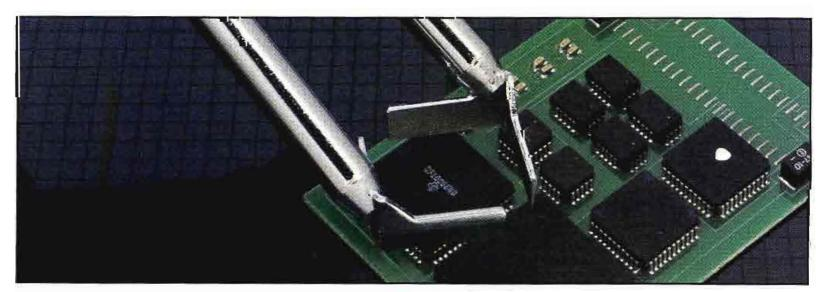
Heated probe tips come in various shapes and sizes. The probe's parallel tips allow all leads of the IC to be heated simultaneously.
