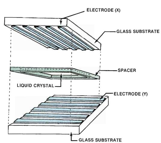
Figure 1. A simple matrix liquid crystal display consists of two glass substrates containing transparent electrodes with liquid crystal material sandwiched between.
