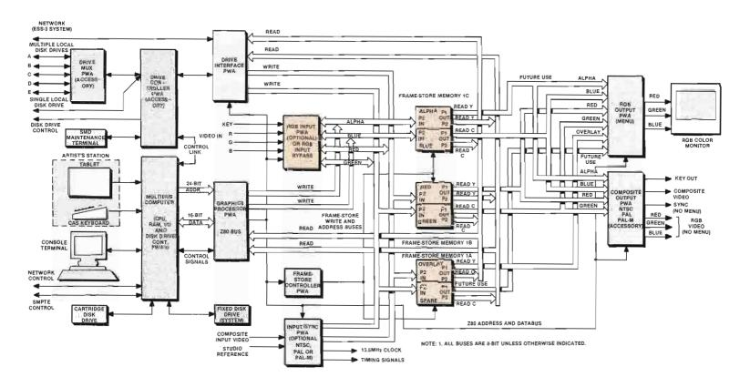
Figure 1. Simplified block diagram of the Ampex AVA-3 video art system.
