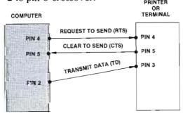
Figure 1. A cable wiring configuration like this is used in many PC-to-printer interfaces.
