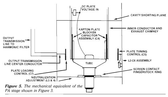
Component C6 is the equivalent stray capacitance between the resistor and the surrounding cavity box.
