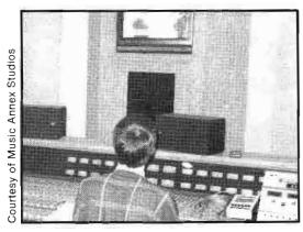
This control room is designed for mixdown work and does not connect to a recording studio. The SMPTE controller, located to the engineer's right, synchronizes the ATR to the edit-master or window-dub videotape.
