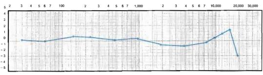
Figure 4. Typical cartridge machine record/play frequency response.
