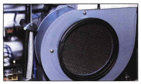
When troubleshooting a transmitter control ladder, don't forget to inspect the operation of the PA compartment air pressure switch and the associated blower assembly (shown here).
