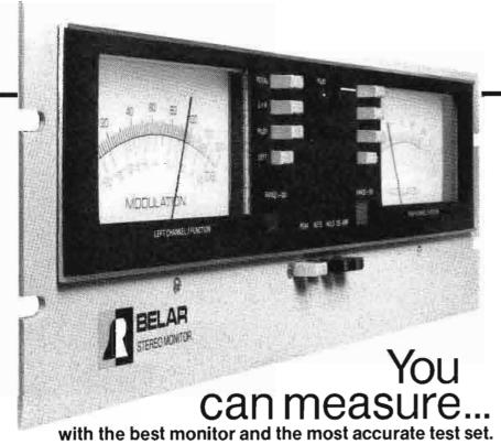
The FMM-2/FMS-2 series monitors provide an even greater degree of precision measurement than ever before... You can measure S/N below 90 dB, You can measure crosstalk below 85 dB, You can measure separations of better than 70 dB, You can measure frequency response to better than **0.25 dB, You can measure** distortions to lower than **0.01%**, and much more... Our uncluttered panels and autoranging voltmeters make these measurements a dream.
