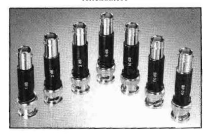
RF Industries has introduced a 1W, BNC in-line, tubular, fully shielded and color-coded attenuator line. The line includes 1dB, 2dB, 3dB, 6dB, 10dB, 20dB and 40dB models. The BNC fittings have gold pins for high conductivity, zero tarnish and low-loss characteristics. The attenuators are for operation to 1GHz and have an accuracy of  $\pm 0.2$ dB to 0.6dB.
