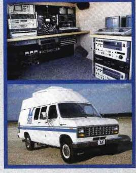
In A Compact, Maneuverable System Midwest utilizes a heavy-duty structural system to combine a 1.8M dual offset-fed antenna with an extended body one-ton van. The result is a powerful satellite communications system that can maneuver easily in city traffic or on narrow country roads.
