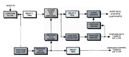
**Figure 3.** An ADM encoder includes delays to compensate for input signal spectral analysis and generation of step and emphasis controls.
