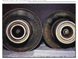
Figure 15. Base heating patterns on two 4CX15,000A tubes. Tube (a), on the left, shows excessive heating and tube (b), on the right, shows normal wear.
