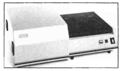
The Tape Care Division of *Data Security* has introduced the Type II degausser, which will erase the 1500 Oersted metal particle videotape used with Panasonic's M-II and Sony's Continued on page 348
