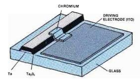
Figure 10. For larger display areas, MIMs are suitable. MIMs can be made using only two or three photo masks.
