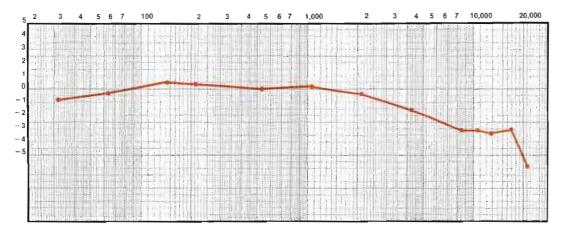
Figure 1. Typical phono cartridge/test record frequency response.
