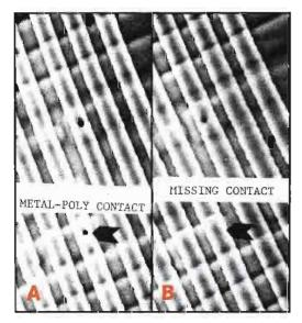
of these interconnects is of critical importance to reliable operation of a device. Figures 6(a) and 6(b) show a failure mode discovered in a common 16K EEPROM device.
