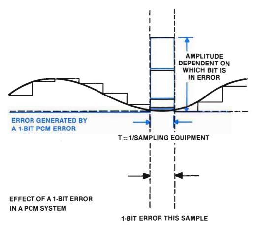
Figure 5. Errors in PCM audio create obvious unusual conditions, while a similar error in ADM coding produces a minimum, self-correcting level offset.
