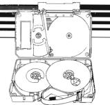
Before we'll reload a ¾" u-matic videocassette we take it completely apart and rebuild it inside and out. We replace wiper flaps, friction pads, tape guides and leader — everything that's needed to make the cassette test as good as new. Only then will we reload it with new 3 M videotapes or other major brands. If we can't rebuild it we won't reload it.
