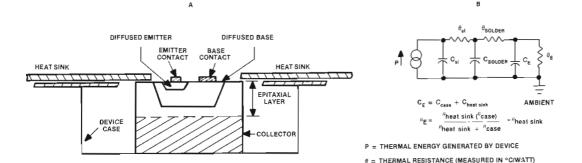
Figure 10. A simplified model of thermal transmission from the junction of a power transistor (TO-3 case) to a heat sink. The structure of a double-diffused epitaxial planar device is shown in (a). A simplified electrical equivalent of the heat transfer mechanism is shown in (b). (Reference 30.)
