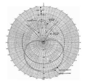
Figure 2. Note the distortion caused in the DA pattern.
