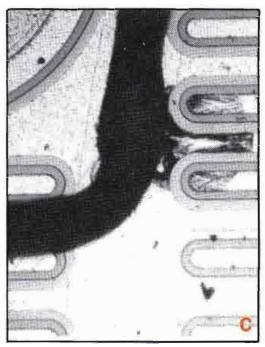
Figure 9. Three views of a hybrid voltage regulator that failed because of a damaged pass transistor. Photo (a) shows the overall circuit geometry. Photo (b) shows a close-up of the damaged pass transistor area. Photo (c) shows an enlarged view of the damage point. (Reference 29.)
