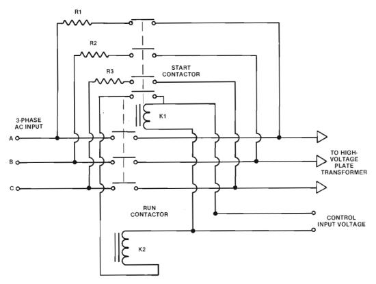
Figure 8. A typical 3-phase step-start power control system.
