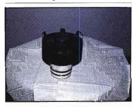
Figure 19. A 4CX10,000D tube that experienced severe overheating. '(Bill Barkley of Econco describes this example as a 4CX10,000D briquet. He suggests that someone stole either the PA blower or the antenna!)
