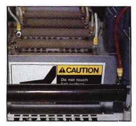
An overheated power resistor often will point to the cause of a power supply fault.
