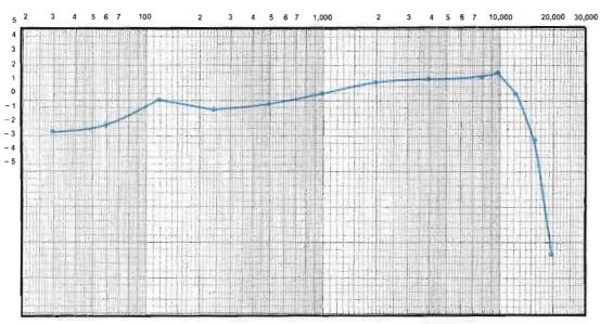
Figure 3. Resulting frequency response measured through the phono cartridge and music equalizer.
