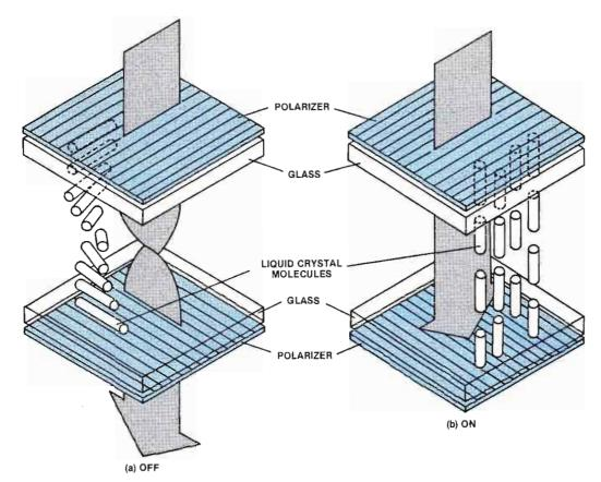
Although there are more than 10 liquid crystal phases, many are not efficient for displays; some are still in development and some are too complex to be costeffective for commercial products. Three types are typically used: dynamic scattering mode (DSM, or simply DS for
