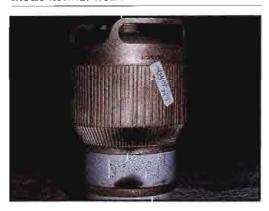
Figure 16. A 4CX5,000A tube that appears to have suffered socketing problems.
