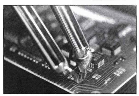
Small components, such as resistors and chip capacitors, can be removed with a parallel-tipped
