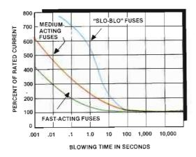
One of the surprising discoveries you will make if you examine literature from fuse manufacturers is that the current rating of a given device is not the brick wall protection value that you may think it is. Consider the graph shown in Figure 28, which illustrates the relationship of rated current across a fuse to the blowing time of the device.
