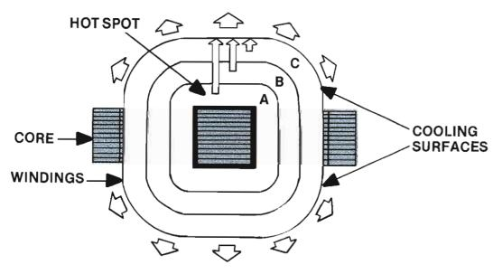
Figure 26. The dynamic forces of heat generation in a power transformer. (Reference 22.)
