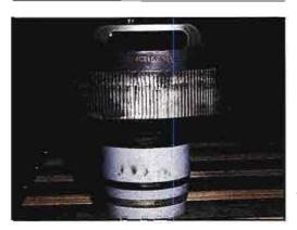
Figure 18. A 4CX15,000A tube showing signs of external arcing.
