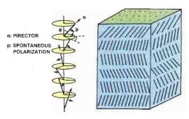
Figure 6. Smectic C liquid crystals have the potential of being ferroelectric and, therefore, suitable for LCDs.
