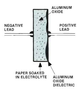
Figure 21. As an aluminum electrolytic capacitor ages, the aluminum oxide dissolves into the electrolyte, causing the capacitor to become leaky at high voltages. (Reference 32.)
