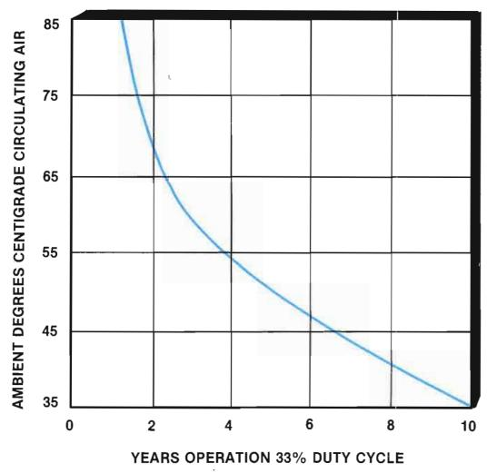
Figure 25. Life expectancy of an electrolytic capacitor as a function of operating temperature.
