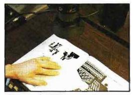
The SpeedTrace function allows any image to be scanned-in to the system with a video camera.
