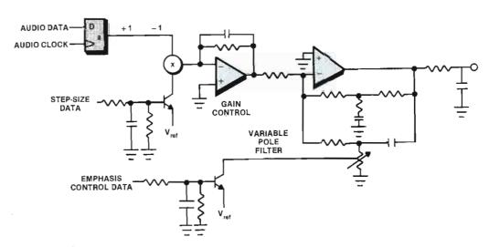
**Figure 4.** Control data, separated by low-pass filtering, provides logarithmic gain control and variable pole control in the de-emphasis network.
