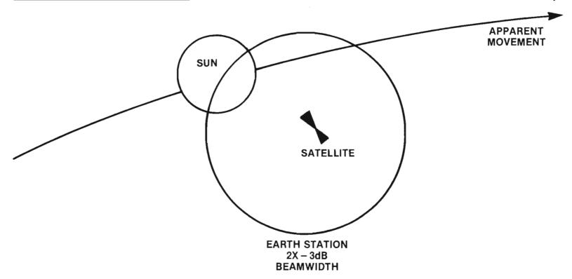
Figure 1. A solar outage is caused by a mini-eclipse of the sun by a satellite. LNA background noise from the sun may obliterate satellite RF.
