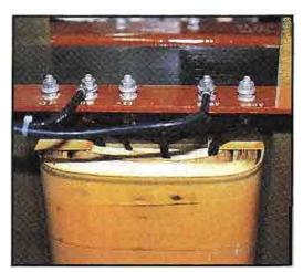
Don't overlook the obvious. Check the tightness of high-voltage and/or high-current cable connections.
