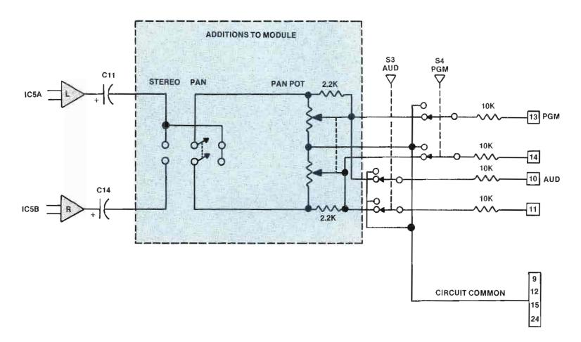
Figure 2. Basic schematic for console modification.
