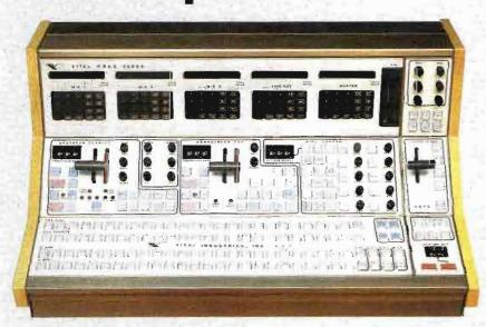
Here's a fantastic switcher with 2, 3 or even 4 Double-Level Mix/Effects systems and occupies only 27" x 18" of console space. This simple ergonomically-designed operations panel can control multiple M/E's at the touch of a button. Yet each M/E of the 3000+ is the same switching powerhouse as the Vital 3000 Series: 2 levels of switching each; an Upstream section that mixes, wipes, title keys and chroma keys, and much more.
